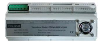
Warning: For cooling purposes the clip-in terminal access panels should be configured like the above image, where air enters from the top left and lower left clip in panels, then exits from fan. All clip in panels should be fitted in this configuration to ensure correct airflow and optimum cooling.
