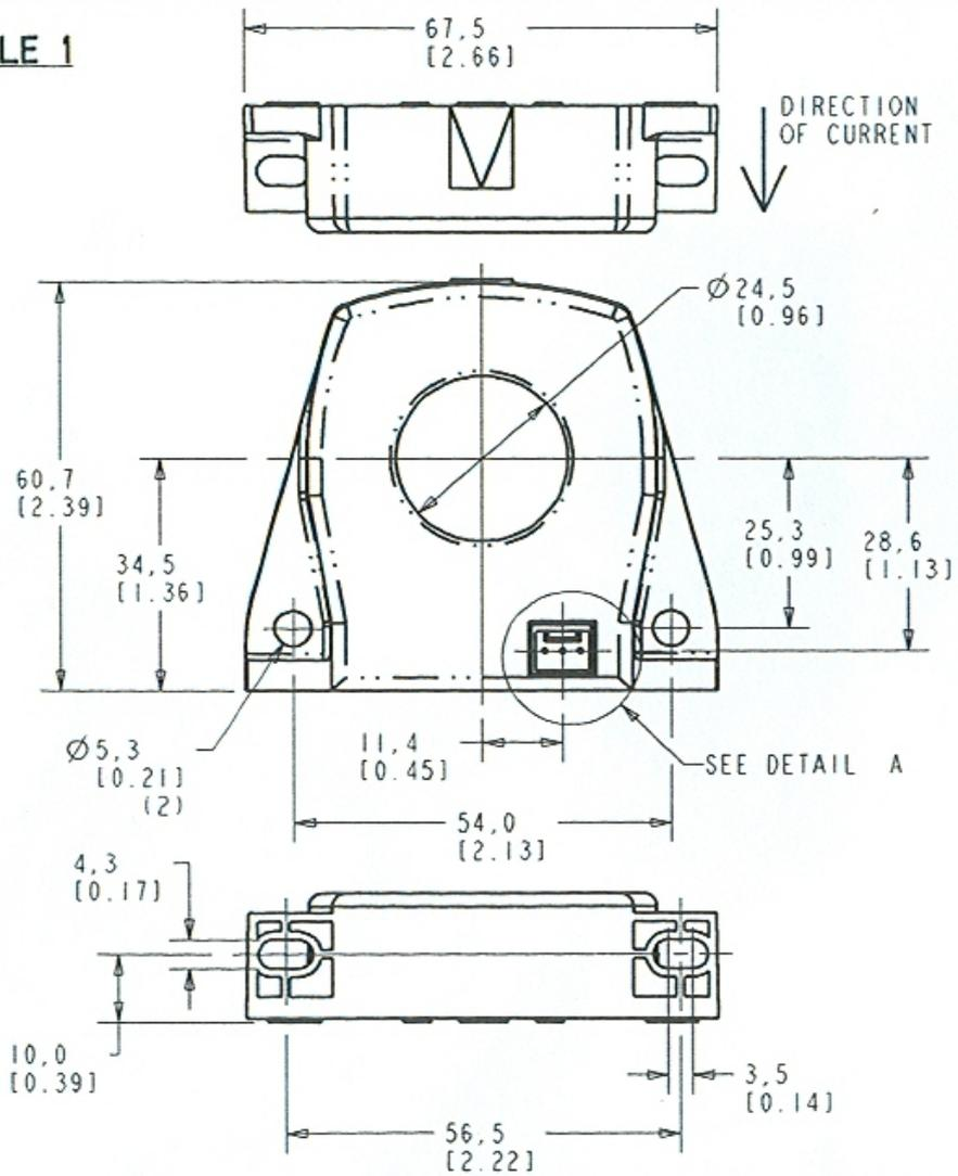
**CTH Current sensor 2" hole - Type 4 (non-split) & Type 8 (split core)**
