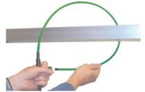
Clip the probe around the dc busbar
