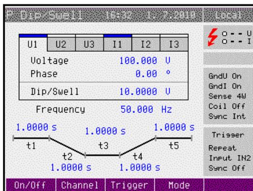
Pressing “Trigger” button starts generation of Dip/Swell shape. Generation can be started (triggered) also from input IN3. Dip/Swell shape is divided into five time periods. Length of these periods can be changed. Active period is during the generation shown in the box.
