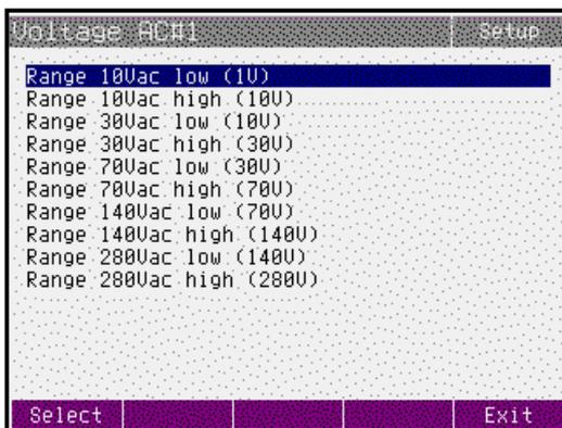
The table lists recommended calibration points. Having selected the required calibration point using Select softkey, the following data are shown.
