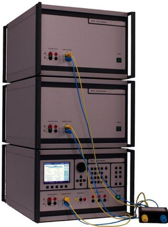
Standard part of delivery the three-phase configuration (1xMC133, 2xMC133f) is the option MC133-01. Using this adapter all current outputs are connected in parallel and the configuration can deliver up to 90 A in single phase mode.
