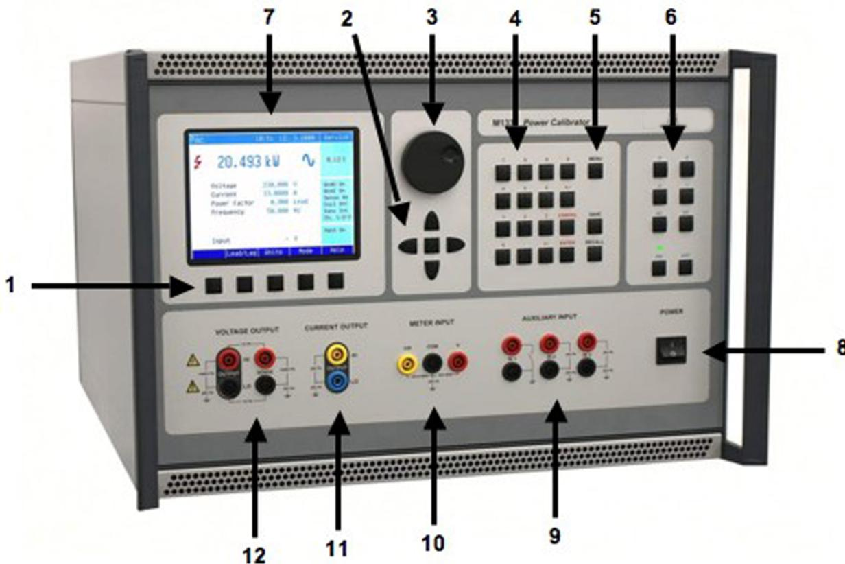
The front panel of the calibrator includes a TFT color display, control buttons and output terminals. The following picture shows the control part of the front panel.
