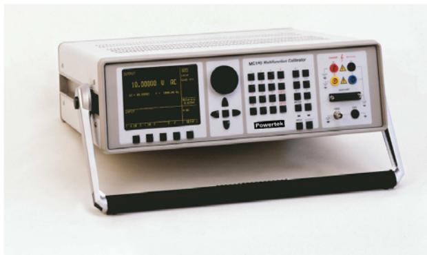
Model MC140 is a bus compatible multifunction calibrator for precise generation of electric units. It is mainly designed for calibration by manufacturers of electronic instrumentation. It also finds its application at laboratories, design and service departments as well as at institutions that have to frequently calibrate their equipment in accordance with their internal quality certification system.
