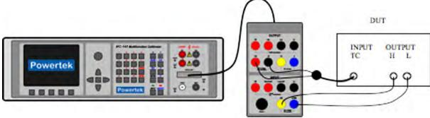
Function setup: Calibrator T RTD function
