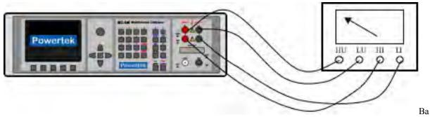
sic connection of a powermeter to the calibrator
