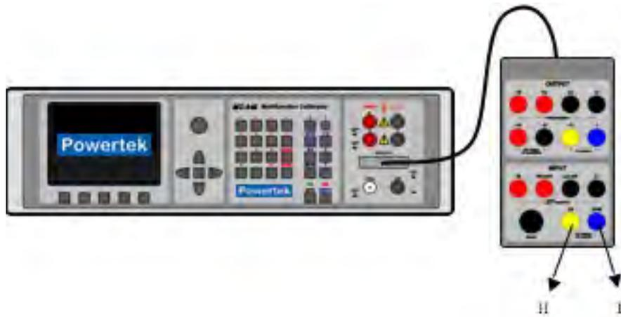
The multimeter allows the measurement of small DC voltages in the range of 0 to 2 V. 140-41 cable adapter is required. The signal to be measured connects to Hu/+mV and Lu/-mV terminals. Lu/-mV is the common terminal of the multimeter. To activate the measurement, select mVDC function mode using METER button in the function menu and press INPUT to measure the input value.
