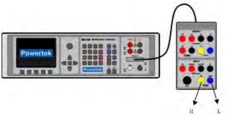
Connection of thermocouple to 140-41 cable adapter:
