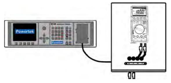
Optional current coil can extend the calibrator's current range to 1000 A. The coil can be used for calibration of both DC and AC ammeters. The clamps of the ammeter must be positioned in angle 90° to the coil. When using the current coil, no steel or other magnetic objects must be present in the vicinity (50 cm) of the current coil, as they would deform the magnetic field and cause big calibration error.
