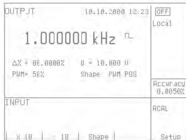
If frequency larger or smaller than the calibrator's range is entered, the calibrator displays an error message: "Value is too large (small)".
