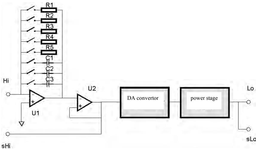
The Hi and Lo terminals are calibrator’s output terminals. The stage including U1 operating amplifier converts voltage to current. U2 is a separation amplifier. R1 to R5 and C1 to C3 are range impedance. DA converter has 0 to +1 and 0 to -1 conversion ration and allows the simulation of resistance and capacitance values different from the range impedances. The output stage increases the permitted current load of the output.
