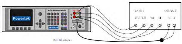
Function setup: Calibrator T TC function
