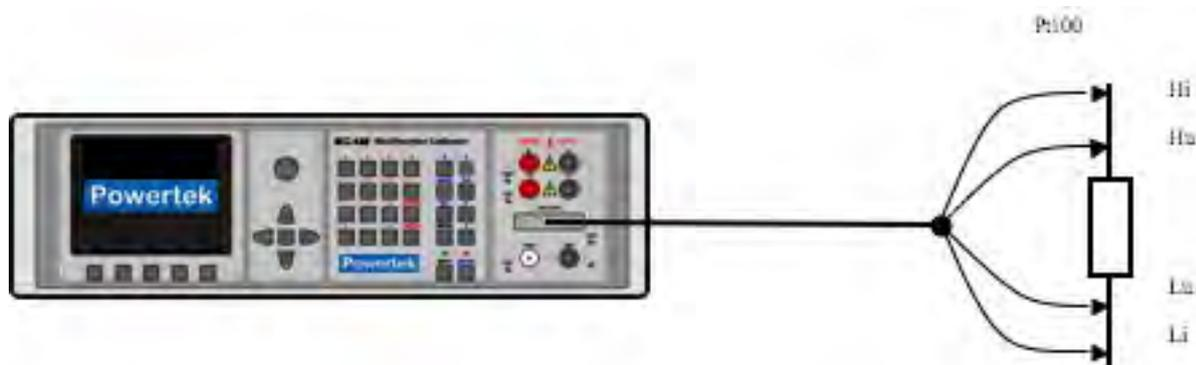
Connection of Pt100 sensor using 140-41 cable adapter
