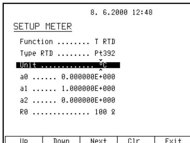
If you want to reset the unit of measurement to original setting, press CLR display button. Original settings are listed below:
