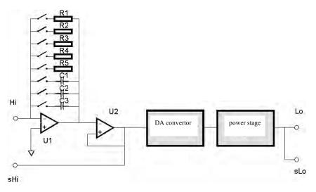
The Hi and Lo terminals are calibrator's output terminals. The stage including U1 operating amplifier converts voltage to current. U2 is a separation amplifier. R1 to R5 and C1 to C3 are range impedance. DA converter has 0 to +1 and 0 to -1 conversion ration and allows the simulation of resistance and capacitance values different from the range impedances. The output stage increases the permitted current load of the output.
