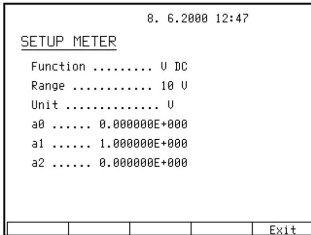
When the multimeter is being set-up, measurement cannot be initiated. Measurement can only be initiated after the menu is left using the INPUT button.
