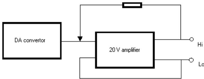
There is a DC reference voltage source integrated within the 22bit measurement converter. Its output is fed to the output stage for 2 and 20 V range. Output voltage present at Hi and Lo terminals is sensed by sensing wires. Feedback eliminates the influence of amplifier's output impedance and of the resistance of wires within the calibrator.
