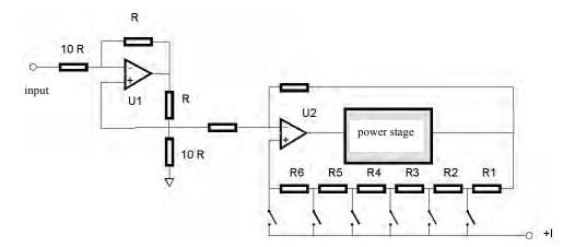
Its input is fitted with overload protection and a separate circuit which measures the shift between output voltage and current in 2 and 20 A current ranges. The output stage is push-pull in B class.
