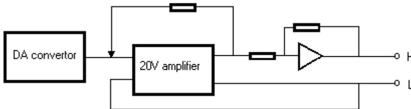
The output of the amplifier is fed to an inverting attenuator with 1:100 nominal division ratio. The signal is then led to the output terminals, sensed via local feedback. This connection allows to load the calibrator output with output current of several mA without losing accuracy.
