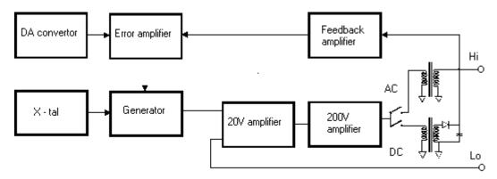
In 1000 V AC mode, the output of 200 V amplifier is transformed and led to the output terminals. The output voltage is sensed, rectified and compared to reference DC voltage provided by the DA converter. error value controls the amplitude of the generator's output so that there is correct voltage at the output terminals. In 1000 V DC mode, 12 kHz signal is transformed, rectified, filtered and led to the output terminals. The output voltage is sensed equally to 1000 V AC mode.
