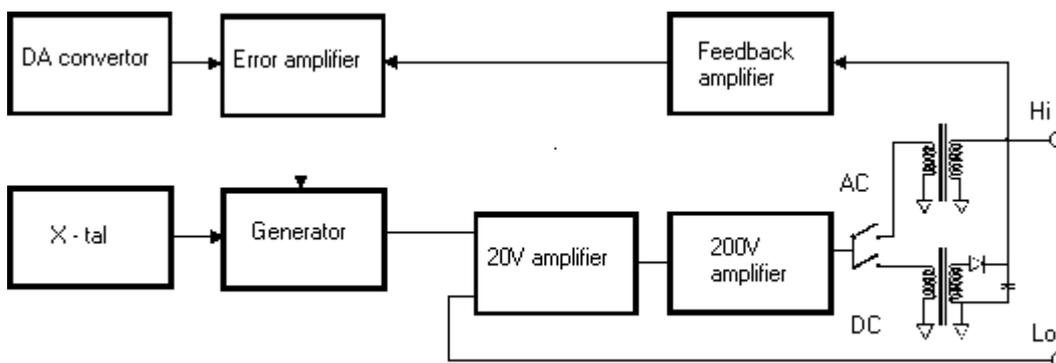
In 1000 V AC mode, the output of 200 V amplifier is transformed and led to the output terminals. The output voltage is sensed, rectified and compared to reference DC voltage provided by the DA converter. error value controls the amplitude of the generator's output so that there is correct voltage at the output terminals.
