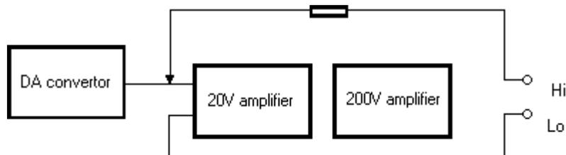
The scheme is similar to 2 and 20 V ranges. A 240 V power amplifier with electronic fuses is connected to the output of 20 V amplifier.
