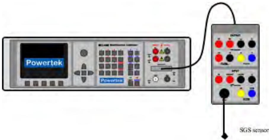
140-41 cable adapter fitted with separate 7pin connector labeled SENSOR is required. The picture shows the connection of the sensor to the calibrator.
