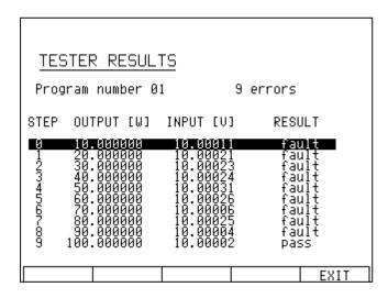
Total number of failed steps is displayed above the table (xx ERRORS) along with the designation of performed test.
