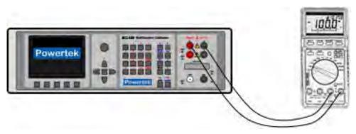
Truncated waveform with defined distortion can be used for testing of multimeters
