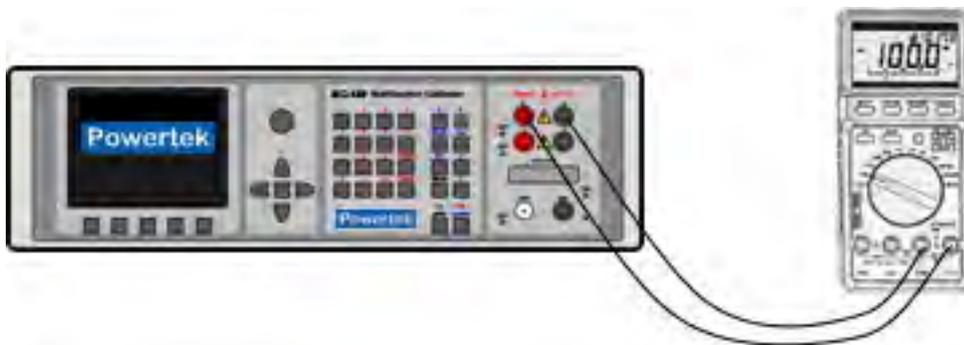
Truncated waveform with defined distortion can be used for testing of multimeters
