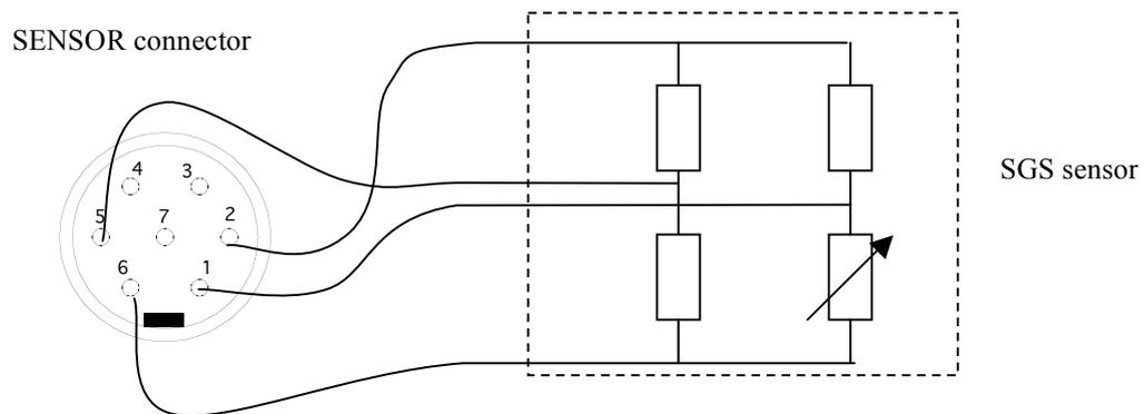
Meaning of pins of SENSOR connector:
