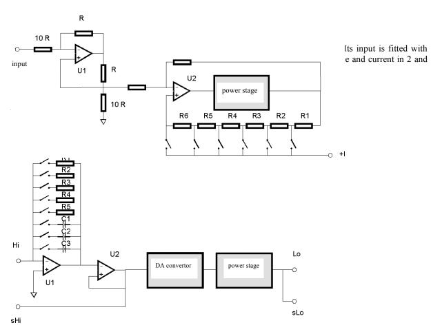
Hi and Lo are calibrator's output terminals. The stage including U1 operating amplifier converts voltage to current. U2 is a separation amplifier. R1 to R5 and C1 to C3 are range impedance. DA converter has 0 to +1 and 0 to -1 conversion ration and allows the simulation of resistance and capacitance values different from the range impedances. The output stage increases the permitted current load of the output.
