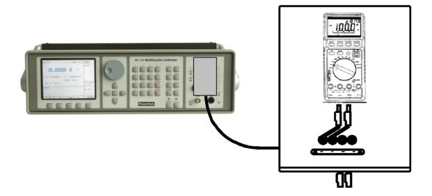
Optional current coil can extend the calibrator's current range to 1000 A. The coil can be used for calibration of both DC and AC ammeters. The clamps of the ammeter must be positioned in angle 90° to the coil. When using the current coil, no steel or other magnetic objects must be present in the vicinity (50 cm) of the current coil, as they would deform the magnetic field and cause big calibration error.
