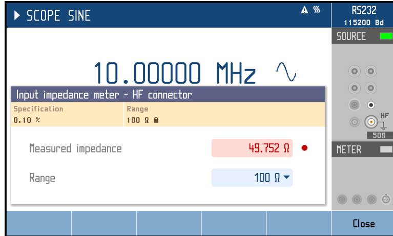
Figure 31 SCO option input impedance measurement
