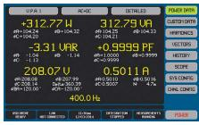
data results (WHr) can also be controlled and viewed from the power data screen. For users with unique data requirements, custom data screens can be built with a spreadsheet application and downloaded to the PA903 via interface or USB drive.
