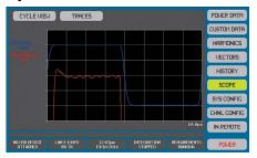
The cycle view represents a single cycle of the voltage and or current periodic waveforms. The above waveforms represent a full 10V square wave in blue and a 50:1 zoomed in view in red. Since the user sets amplitude and scaling - the result is an almost unlimited ability to amplitude zoom to expose fine detail. The sampling is forced to be asynchronous to higher order harmonics which leads to an effective sampling rate of 384MSPS.
