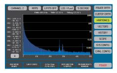
Additionally, eight harmonics can be selected for numeric display of amplitude and phase by touching the harmonic bar of interest. The user may also import harmonic limits, which when enabled will show out of tolerance harmonics in red above the limit line.
