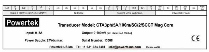
CTA3ph and CTV3ph three phase Integrator signal conditioner - product label will depict the function of each terminal. CTV3ph units do not use an output transformer
