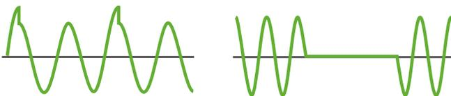
Transient generation is an extended feature that provides the users an easy setup for power line disturbance simulation. Common waveform disturbances such as surge, sag, spikes, and dropouts can be generated for application like immunity test.
